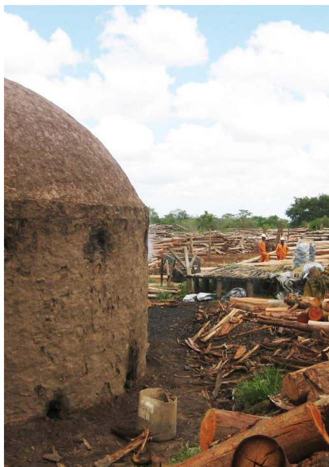
Different kiln types with efficiency rates of 28-30%. More advanced high-end kilns have efficiency rates of up to 75%. Iiyama M, Neufeldt H, Dobie P, Jamnadass R, Njenga M, Ndegwa G (2014) The potential of agroforestry in the provision of sustainable woodfuel in sub-Saharan Africa. Current Opinion in Environmental Sustainability. Vol. 6C, pp. 138-147. http://dx.doi.org/10.1016/j.cosust.2013.12.003 . Photo 1: Valter Ziantoni/ICRAF Photo 2: with metal kiln Miyuki Iiyama/ICRAF
